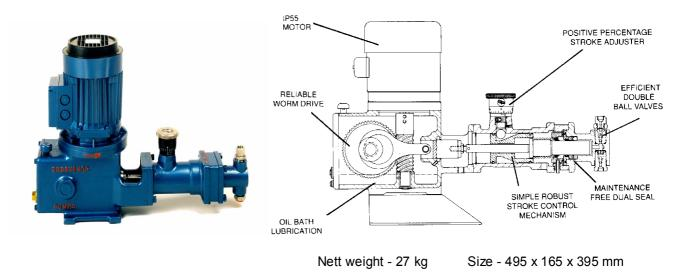
The Pygme Variflow pump is a variable output single acting plunger pump with high efficiency double ball valves. Drive from vertical flange mounted motor is through a worm and wheel to the eccentric which operates a push rod. This rod actuates the robust and trouble free spring return adjusting mechanism which is fitted with a manual micrometer adjusting screw. The stroke length is adjustable 0 - 100%.
