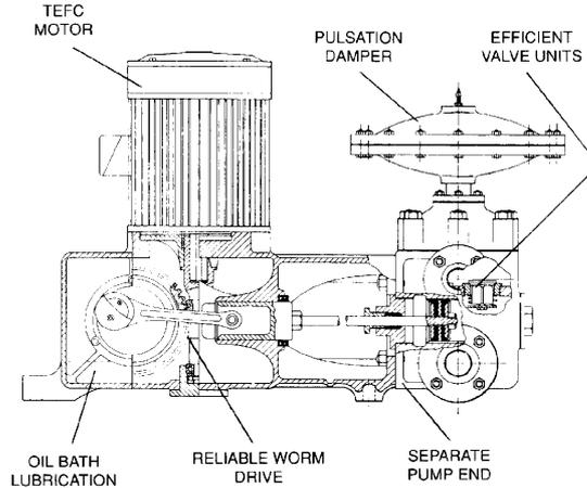
Weight (Typical) 275kg Size (Typical) 730 x 400 x 700mm
