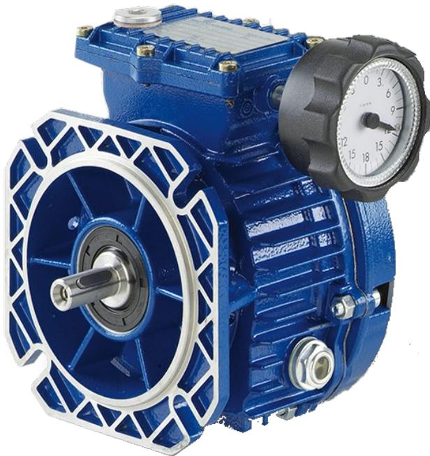
Motovario Disc Variators operate on a sun race & planet gear assembly. Two sun races (1&2) are pushed together via a set of Belleville springs (3) and are keyed to the input shaft (4).
