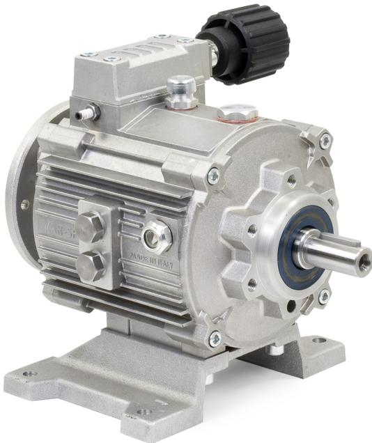
Var-Spe infinitely variable hydraulic gears work according to the principle of hydrostatic transmission. They essentially consist of a hydraulic, radial piston variable displacement pump (primary pump) and a constant displacement pump (secondary pump).
